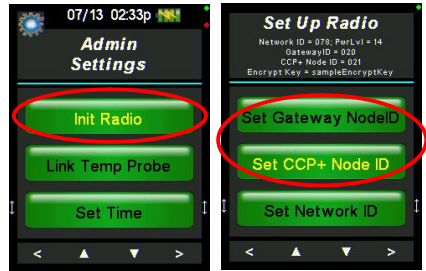
Figures 6 & 7: Clicking Init Radio brings you to Set UP Radio
