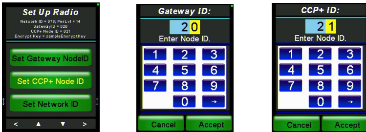
Figure 51: Initializing the Radio by setting the Gateway and CCP+ ID's.
