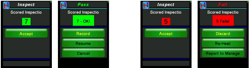
Figure 29: Two inspection examples (left) Inspection score passed. Press Record to continue. (right) Inspection score failed. A screen follows with corrective actions.
